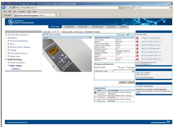
MONITOR UP TO TEN PUMPS WITH ONE CIU27X MODEM
